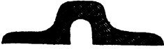
Fig. 160—Represents a cross section of the rail of the Great Western Railway in England. This rail is laid on a continuous support, and is fastened to it by screws on each side of the rail. A piece of tarred felt was inserted between the base of the rail and its support.
